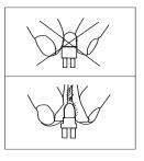
This fixture is fitted with a discharge lamp which are highly susceptible to damage if improperly handled. Never touch the lamps with your bare fingers as the oil from your hands will shorten lamp life. Also, never move the fixture until the lamps have had ample time to cool. Remember, lamps are not covered under warranty conditions.
