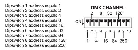
Dipswitch 10 is used to control the Master/Slave operation. Turning dipswitch 10 on will activate that unit as a "Master Unit."
